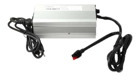
**The Exodus Model LL-14615A,** 14.6VDC, 15A AC-to-DC Charger, is an AC-to-DC charger for use in charging 12V LiFePO4 batteries. This charger has an Anderson Powerpole plug or Alligator Clips for charging Exodus 12V Batteries. Please ensure that the LiFePO4 batteries include a PCM/BMS when using this particular charger.
